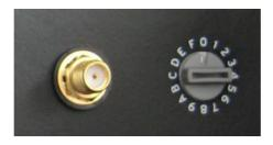
Transmitter and receiver must be set on the same frequency.
