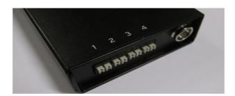
To connect the effects press the connector, the contact will open and effect can be connected.
